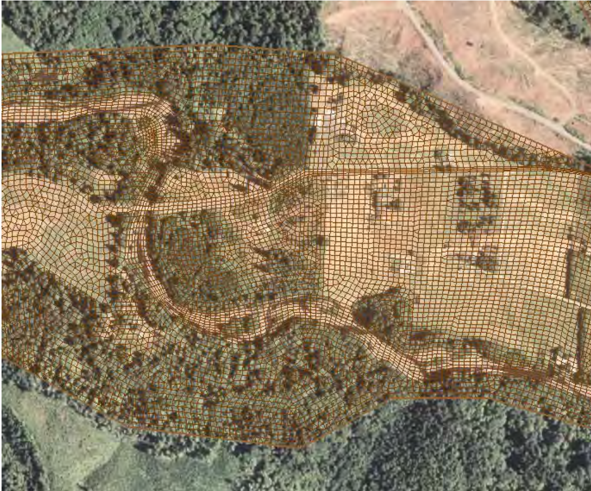
Figure 12. Example of 2D model mesh along Vance Creek.
